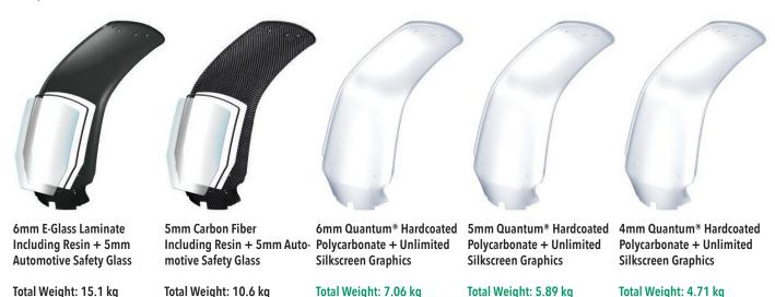
Since hardcoated polycarbonate is so much stronger and more impact resistant than safety glass, you can substitute 4mm polycarbonate glazings for what were considered the norm with 5-6mm glass – with less than 1/3 the normative weight.
